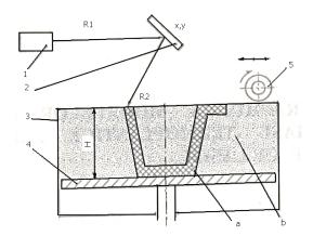
Fig. 1. Laser sintering operation is shown schematically in figure 1 - laser, 2 - scanner, 3 - tank, 4 - mobile platform, 5 - smoothing and drying system, R1, R2-ray laserpart consists of b-powder.
